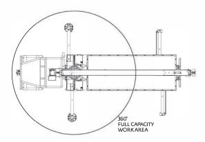
The mounting configuration is based on an 85% stability factor. If the bare truck weight requirements are not met, counterweight will be required. The complete unit must be installed on the truck in accordance with factory requirements. Since individual truck chassis vary, a test must be performed on the unit to verify actual stability after mounting and counterweighting (if required). A summary of mounting and truck requirements are:
