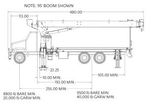
**Note:** Chassis will require extended front frame rails for SFO addition.
