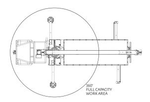
The mounting configuration is based on an 85% stability factor. If the bare truck weight requirements are not met, counterweight will be required. The complete unit must be installed on the truck in accordance with factory requirements. Since individual truck chassis vary, a test must be performed on the unit to verify actual stability after mounting and counterweighting (if required). A summary of mounting and truck requirements are:
